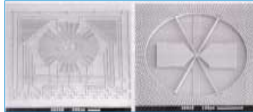
Detail of the silicon-based accelerometer developed under Si-Gyro
